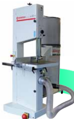
MM-EXTRACTION70 shown fitted to MM-BANDSAW13 with adapters supplied in MMP-EXT-CONKIT1
