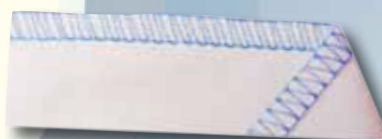
3 thread overlock 5mm
