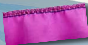
Gathered edge using the differential feed
