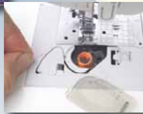
Drop in bobbin with easy to use thread guide
